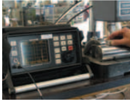
Quality assurance Ultrasonic testing
